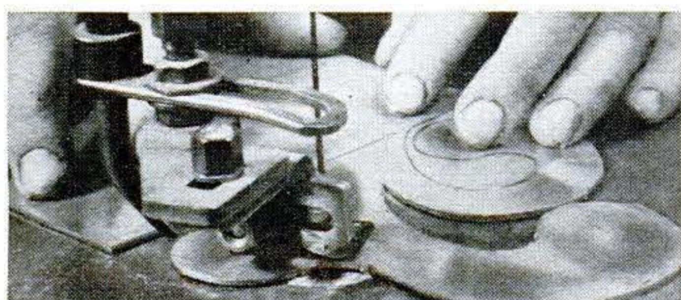
Cut the copper to shape on a jigsaw, or if this is not available, a jeweler's saw may be used.
